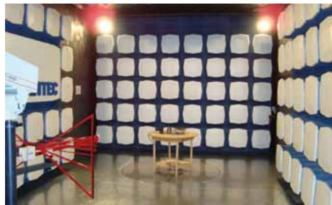
PRODINTEC provides counselling to companies on the legislation framework in force in terms of electromagnetic compatibility and CE marking, as well as on the design of electrical and electronic products, focusing on the final compliance of the norms. We also have a fully equipped laboratory (shared with the University of Oviedo) to carry out compatibility tests.
