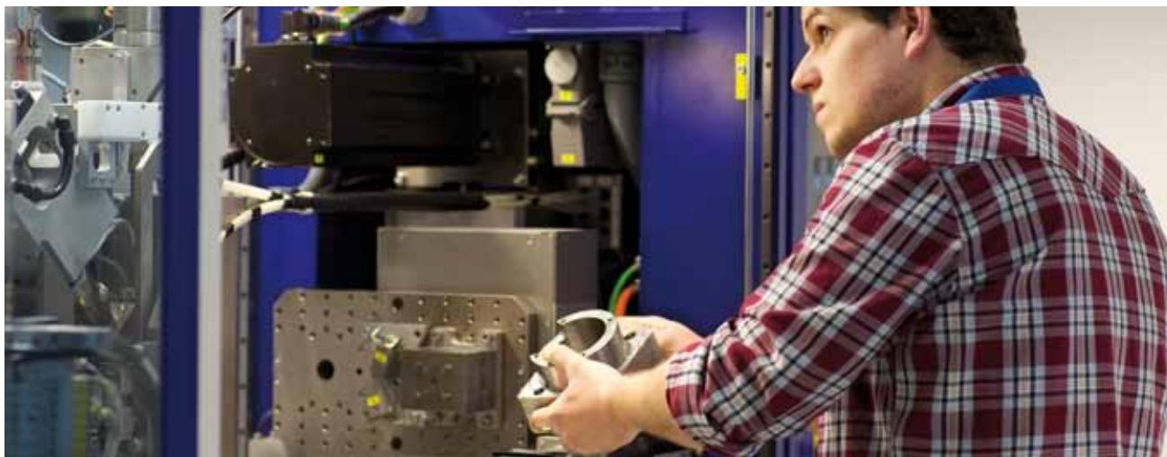
We also have a high-speed 5-axis milling machine that allows us to produce very high precision parts with complex geometries in any material: up to HRC 65 steels, stainless steels, aluminium, copper, bronze, brass, molybdenum, super alloys, plastics, resins, ceramic materials, wood, etc.
